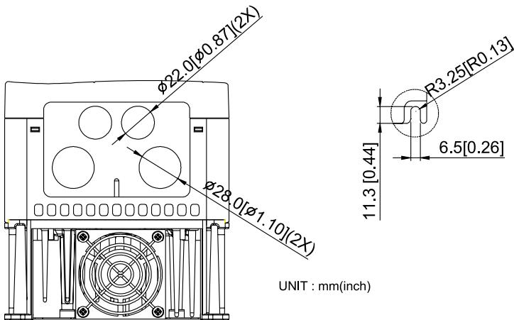
Типоразмер С: VFD055B23A/43A/53A, VFD075B23A/43A/53A, VFD110B23A/43A/53A
