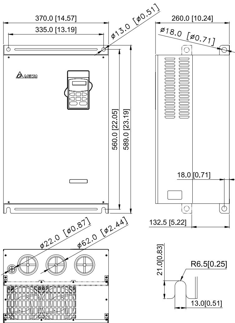
Типоразмер Е1: VFD300B23A, VFD370B23A, VFD550B43C/53A, VFD750B43C/53A
