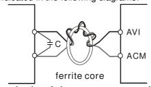
wind each wires 3 times or more around the core
