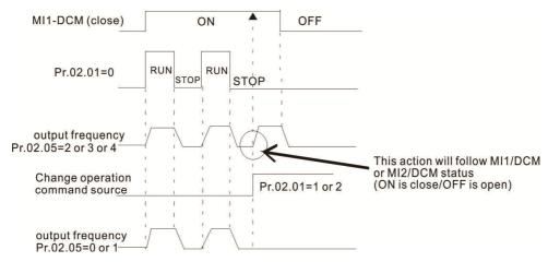
The Line Start Lockout feature does not guarantee that the motor will never start under this condition. It is possible the motor may be set in motion by a malfunctioning switch.
