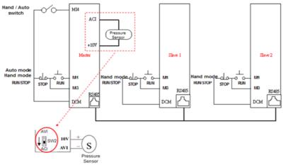
Wiring of the pressure sensor:
