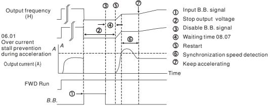
Fig3: B.B. Speed Search with Minimum Output Frequency Upward Timing Chart
