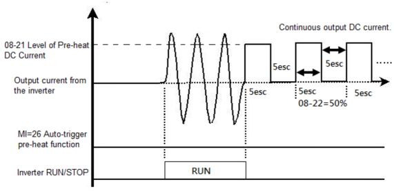
The figure below shows the Sequential Relation between Pre-heat function & enabling DC brake.
