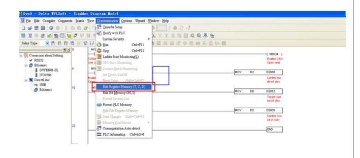
Click Transmit, and choose D1070~D1099 D2000~D2799, and click the "Read from PLC Device Register" for reading the D1070~D1099 D2000~D2799 from Current PLC.
