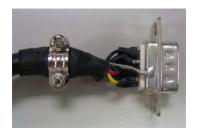
(1) Solder the centre cores on the metal part of the connector adequately for good ground contact with the plate and shielding.
