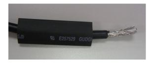
Cut through the cable and expose the core wire which covers the metal core wires with shielding. The reserved core wire length should be 20~30mm. Then, cover a 45mm heat shrink tube on the cable.
