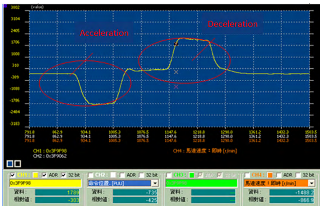
Figure 3.5.16 Monitoring Position Deviation of Gantry
