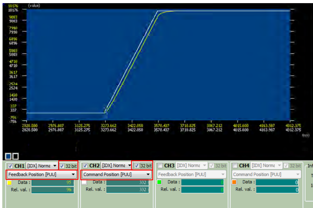
Figure 1.39 Monitoring Variables on PC Scope (32-bit)
